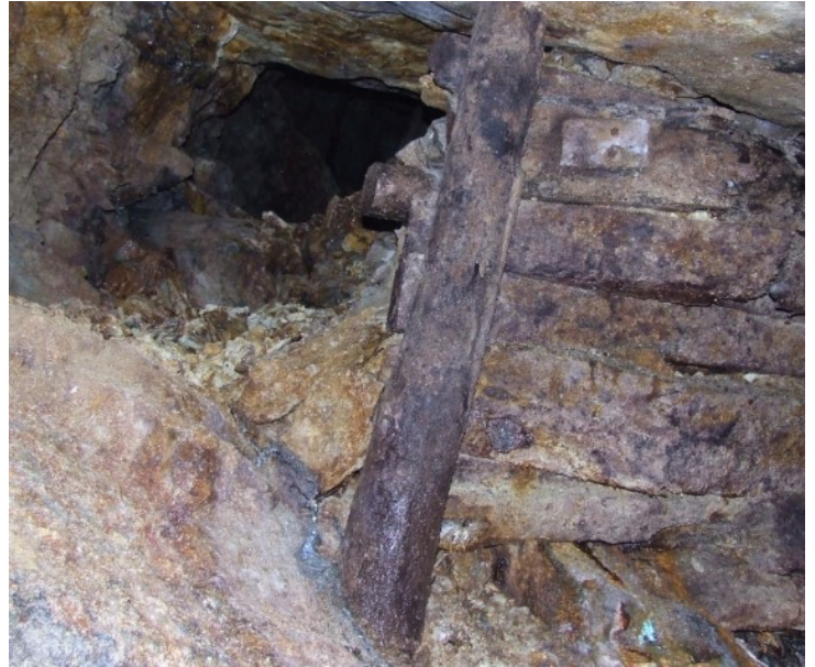
Figure 660: (left) Opencast workings at Prince Edward mine. (right) Underground stope working on the mineral lode, which dips at 70^{\circ} at this point.
